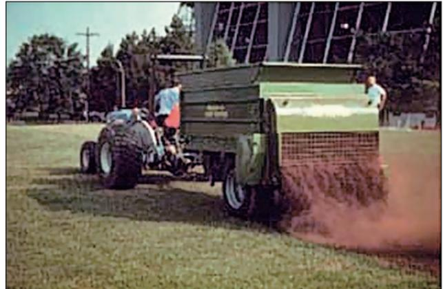
**Figure 5:** Modified spreaders with conveyer belts and brushes mounted on the back are ideal for surface applications of SMS.
